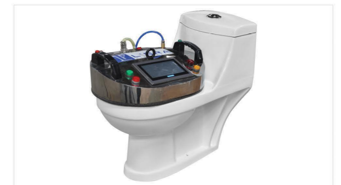
One Piece Tested By Vacuum Machine
